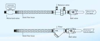
Hose kits are provided as a set according to model/flow rate of heat pump.
